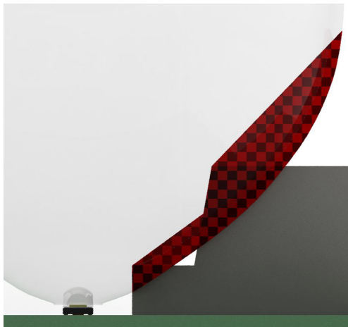
Figure 5: Red checkered pattern indicates light blocked by components near the LED
