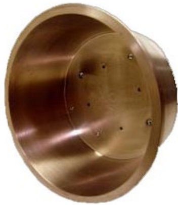
Figure 3: Custom-made aluminum housing
